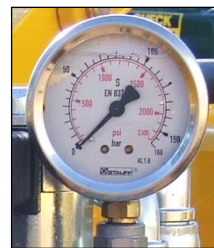
Accumulator Pressure Gauge
